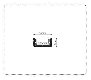
$\mathsf{XS}1608$  Premium extrusion comes complete with plastic end caps and an opal frosted diffuser.
