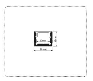
Premium extrusion comes complete with Aluminium end caps and Opal Frosted diffuser. Use XS1613 extrusion for flawless dot free light compared to ultra-shallow extrusion.
