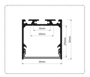
Premium extrusion comes complete with Aluminium end caps and opal frosted diffuser.
